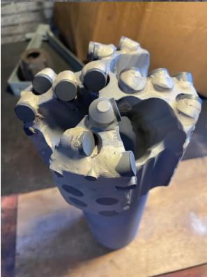
Stick Pipe reverse circulation 8,120 ft of abrasive fill and scale in 53 hours. In gage and refit with two new cutters.
