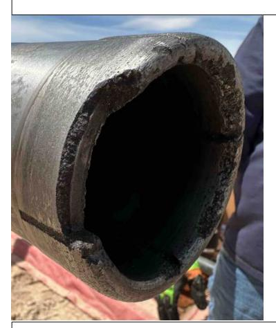
Note: Excess WOB belled the matrix and cracked
