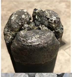
Many (estimated 12) carbide mills run to drill 120 feet of drill pipe with last piranha mill making NO new headway (stopped on tool joint).
