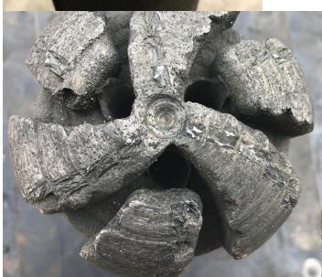
3 7/8" MX-C was ordered/ fabricated/and in the hole within 24 hrs and made a total of 98 feet to finish the job. As you can see the carbide inserts were not lost downhole even though they are completely shattered
