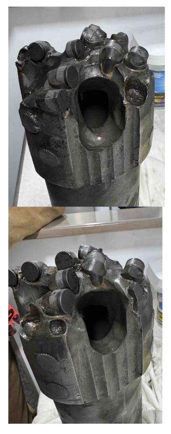
Reverse Circulating PDC Mill Steel Body with 13mm PDC discs mounted on 1/2" Steel Posts
