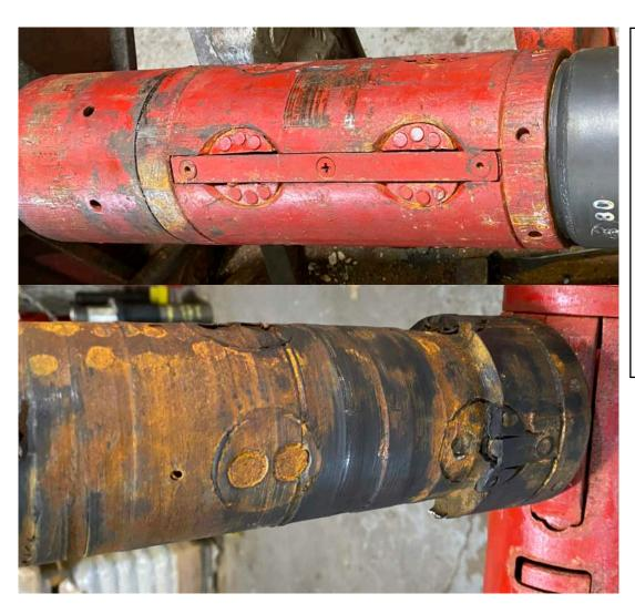
Prior to running the XDS diamond shoe there were several (2-3) WC shoes that could not cut the first set of four strap-set Slip Block that held six 3/8" Carbide Slip Buttons.
