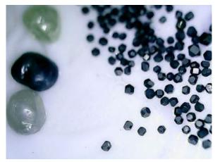
Shown at far left are three grades of processed/conditioned mined diamonds that are sized 6-8 stones here carat that measure about .100" diameter. These are set in raised matrix ridges to increase their effective exposure/standoff while protecting them from impact loads that can fracture them.
