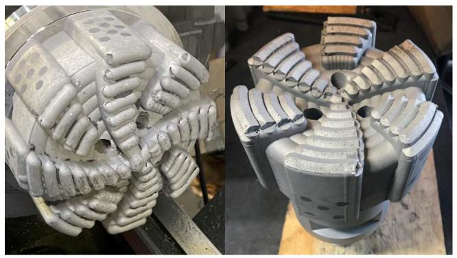
These mills can be custom sized and shaped tp fit your extreme targets. The "blades" are raised 1/2" or more from the mill face where WC carbide inserts are set in the leading edges of each diamond "Pod" that is filled full height with 30-40 mesh diamond grit that is held in place by the furnace infiltrated Matrix (not torch-made). The inserts become an integral part of the matrix and cannot be lost out of the mill face even when fractured.
