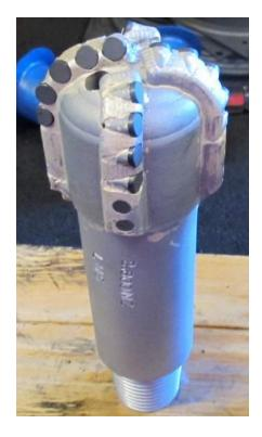
Above is a 2.500" MZ-54 set with 8mm PDC and maximum junk slot area and gage pads set with 10mm TSD and rounded edges for minimal free rotating torque.
