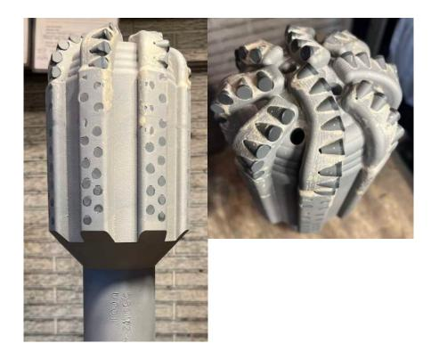
Above is a 5.500" MZ-48G 8 blades set with 10mm PDC's with an extended gage with rounded edges for minimal free rotating torque. Face with six directed fluid ports.
