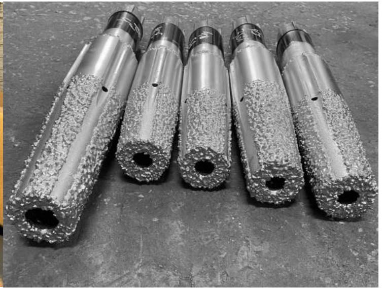
Options shown above are Extra Thickness of 1/4" Starbide chips set with massive pad shape with a closed center and large chip up drill
