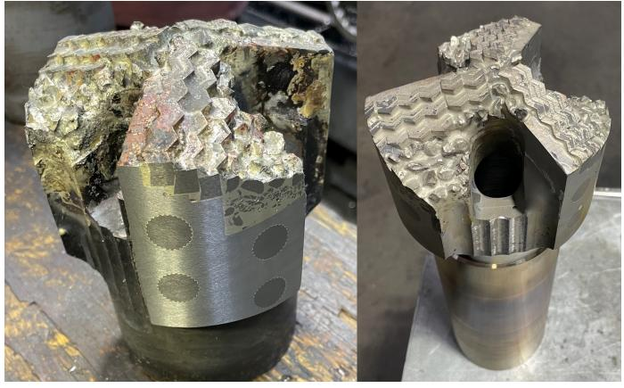
Hard-Set Chevron Inserts Reverse Clutch Three Large 1" Reversing Ports = 2.36 TFA 2 7/8" PH-6 Box With 2" Bore = 3.14 area
