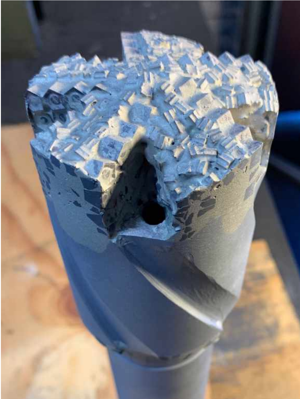
SK (convex)(closed center cut) Patriot 5 side WC Inserts Reverse Spiral Gage WC Updrill
