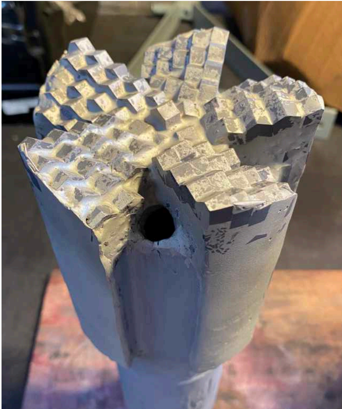
Custom SKK-RC Reverse Clutch With Chevron WC Inserts
